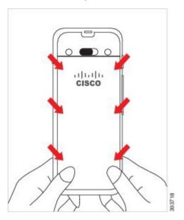
**Caution** Do not force the cover. If it doesn't click into place easily, remove the cover and check that the battery is inserted correctly.
