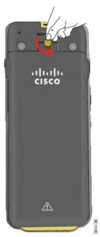
**Caution** Don't use a sharp object to unscrew the battery compartment door or to pry the battery door off the phone.
