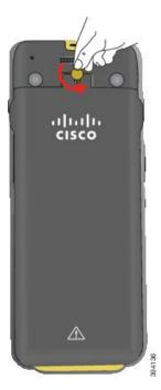
**Caution** Don't use a sharp object to unscrew the battery compartment door or to pry the battery door off the phone.
