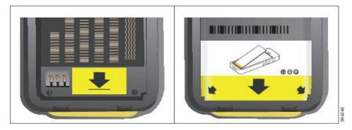
a) Hold the battery so that the lower edge is close to the bottom of the compartment. Make sure that the metal contacts on the phone and battery face each other. On the battery, the Cisco logo must be near the locking catch and the arrow must point to the base of the phone.
