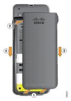
**Caution** When you close the battery cover, make sure that it is completely closed. Otherwise dust and water can enter the battery compartment.
