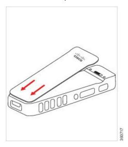
b) Press the cover firmly against the phone until it clicks in place. Press at the top, middle, and bottom of the cover on each side.
