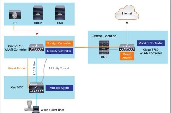
The topology shown in Figure 1 represents a Cisco Catalyst 3850 access switch that is acting as a mobility agent where guest users plug in directly on the access port. The corresponding mobility controller is the Cisco 5760 WLC, local to the site. The local Cisco 5760 WLC connects to another Cisco 5760 WLC at the central location that acts as the guest anchor. The guest tunnels terminate on the guest anchor.
