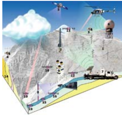
FIGURE 1. A typical data source context for next-generation environmental science, with a heterogeneous sensor deployment that includes (1) mobile stations, (2) high-resolution conventional weather stations, (3) full-size snow/weather stations, (4) external weather stations, (5) satellite imagery, (6) weather radar, (7) mobile weather radar, (8) stream observations, (9) citizen-supplied observations, (10) ground LIDAR, (11) aerial LIDAR, (12) nitrogen/methane measures, (13) snow hydrology and avalanche probes, (14) seismic probes, (15) distributed optical fiber temperature sensing, (16) water quality sampling, (17) stream gauging stations, (18) rapid mass movements research, (19) runoff stations, and (20) soil research.
