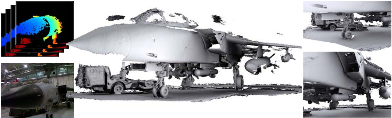
Figure 1: We take depth maps from a consumer depth camera (top left) and fuse them into a single surface model (center & right) in real-time using a compact GPU data structure. This allows live reconstruction of large-scale scenes with fine details (rendered w/ ambient occlusion).
