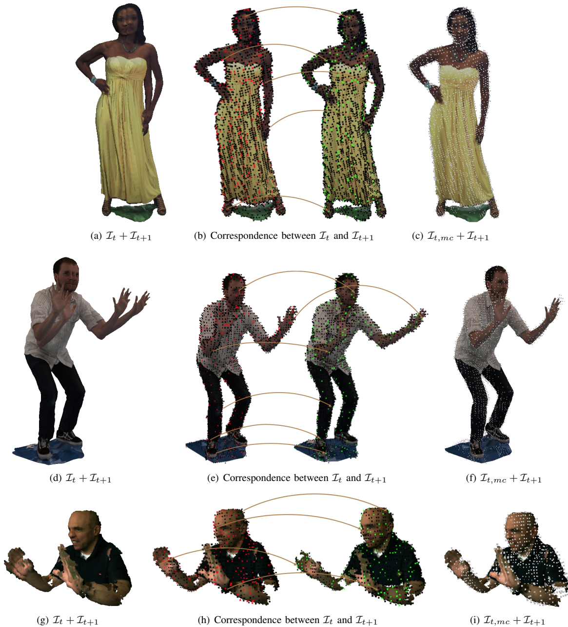
Fig. 9. Example of motion estimation and compensation in the yellow dress, man and upper body motion sequences. The superimposition of the reference ( \mathcal{I}_t ) and target frame ( \mathcal{I}_{t+1} ) is shown in (a), (d), and (g) while in (b), (e), (h) we show the correspondences between the target (red) and the reference frame (green). The superposition of the motion compensated reference frame ( \mathcal{I}_{t,mc} ) and the target frame ( \mathcal{I}_{t+1} ) is shown in (c), (f), and (i). Each small cube corresponds to a voxel in the motion compensated frame.
