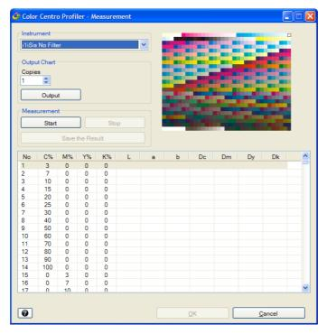
From [Instrument], select the instrument to use for the measurement.
