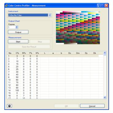
3 From [Instrument], select the instrument to use for the measurement.
