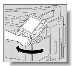
Do not grab the touch panel when turning the control panel to the left or right.
