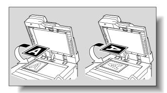
Align the original with the mark in the back-left corner of the original scales.
