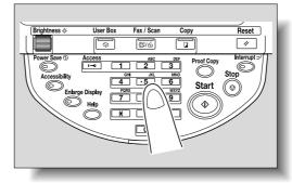
If the number of copies was incorrectly entered, press the [C] (clear) key in the keypad, and then specify the correct number of copies.
