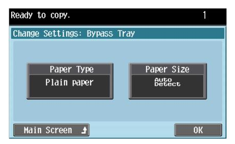
4 Select the appropriate setting for the type of special paper that is loaded. Touch the button for the desired paper type.
