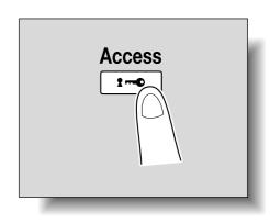
When you are finished performing the desired operations, press the [Access] key. A message appears, requesting confirmation to log off.
