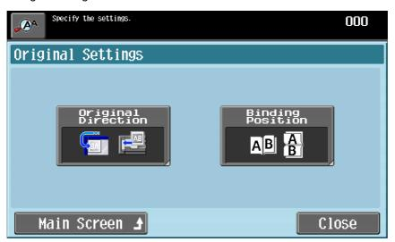
Touching [Original Direction] displays the Original Direction screen. Touch the button for the desired orientation, and then touch [OK].
