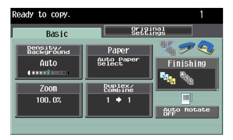
3 To return to the standard-sized screens from the screens in Enlarge Display mode, press the [Enlarge Display] key in the control panel.
