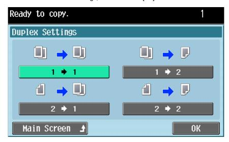
If "1 > 2" or "2 > 2" is selected, touch [Output Bind Direction], select the binding position for the copy, and then touch [OK].
