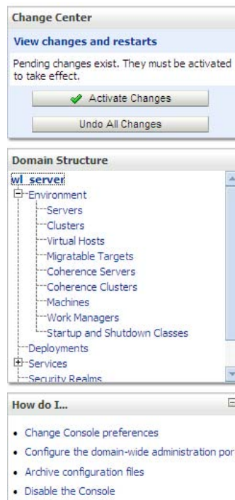
FIGURE 1-5. The Activate Changes button in the Change Center
