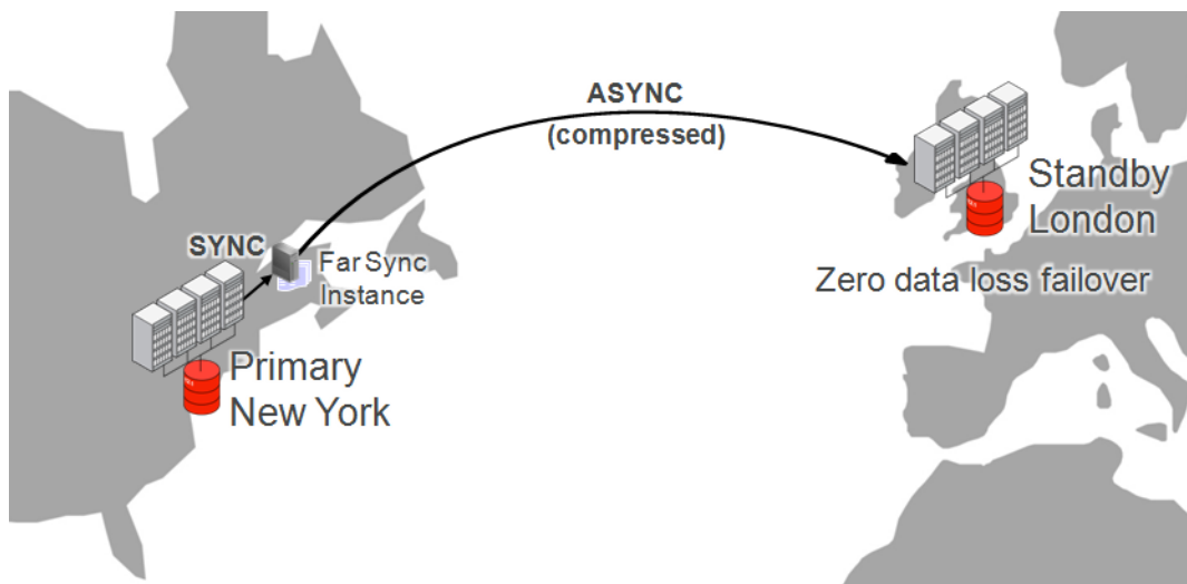
Figure 3: Active Data Guard Far Sync – Zero Data Loss Protection at any Distance
