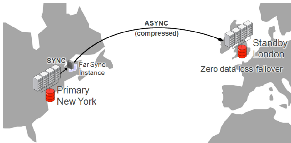
Figure 2: Active Data Guard Far Sync – Zero Data Loss Protection at any Distance
