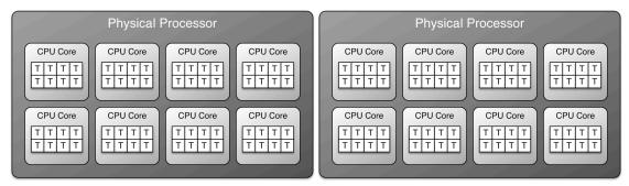
Figure 1: A system with 2 processors, 8 cores per processor and 8 threads per core
