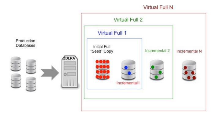
ZDLRA indexes all backups creating a pointer-based representation that stores the corresponding metadata within its catalog. During restore, the appliance constructs a virtual full backup to the point of the incremental which is then sent to the database server along with any necessary archived log backups for point-in-time recovery. The virtual full restore capacity gives users the same level of service as if a daily full backup had been performed, without the overhead or performance impacts.
