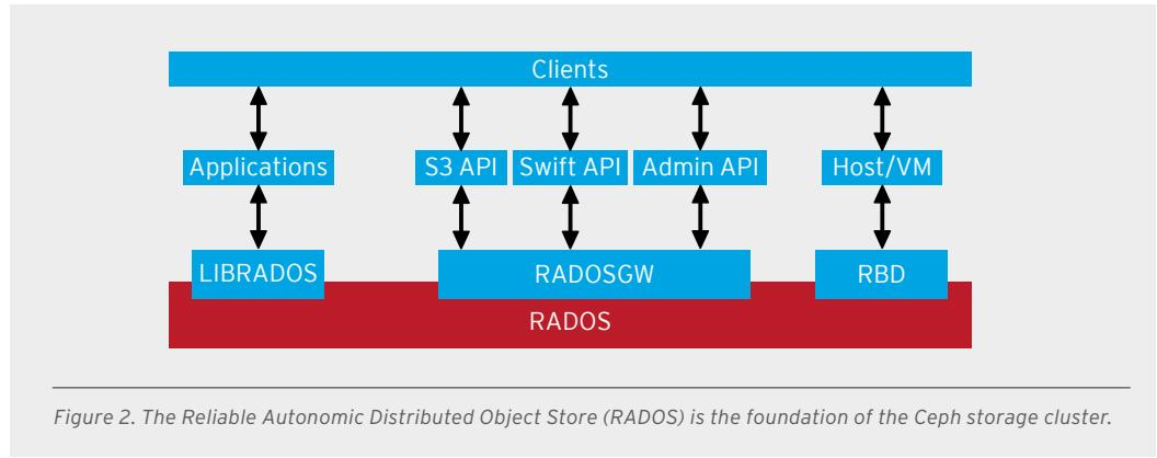
Writing and reading data in a Ceph storage cluster is accomplished using the Ceph client architecture. Ceph clients differ from competitive offerings in how they present data storage interfaces. A wide range of access methods are supported, including:
