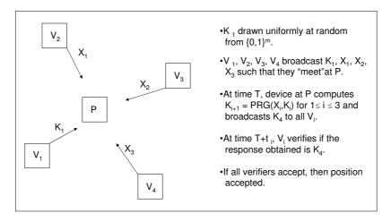
Figure 1: Secure positioning protocol in 3-Dimensions
