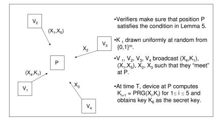
Figure 2: Position based key exchange in 3-Dimensions
