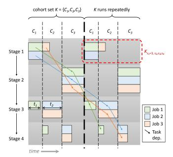
Fig. 3. Cohort Scheduling Example, n=4 stages. The cohort set K which starts j=3 jobs consists of cohorts  $C_1=\langle 2,0,1,0\rangle,\ C_2=\langle 1,0,2,1\rangle$  and  $C_3=\langle 0,3,0,2\rangle$ . Two sequential executions of K are shown.
