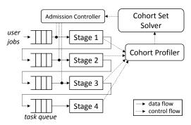
Fig. 2. Host Scheduler. Admission controller gates the number of tasks that are permitted to run. The gate policy is set by the Cohort Set Solver, which is in turn fed data by the Profiler.
