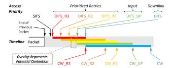
Fig. 4. Wireless Scheduler's Low Latency 802.11-compatible MAC. Input and its retries receive priority over video downlink traffic. Colored bars represent the time window of opportunity to acquire the channel.
