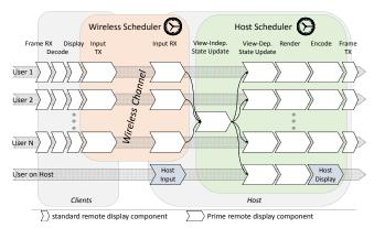
Fig. 1. The Prime Framework. Clients connect directly to the Host using Wi-Fi. Apps are executed as dataflow. Prime's Host and Wireless Schedulers optimize the dataflow for latency, throughput and fairness.
