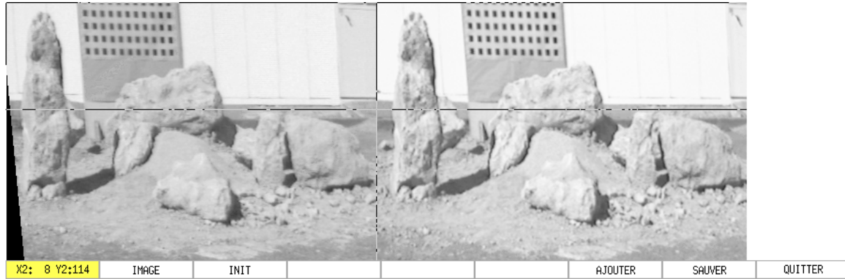
Figure 3: Rectified stereo pair
