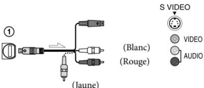
Câble de raccordement A/V (fourni)
