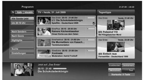
Figure b: EPG application, broadcast video is shown on the left bottom, can be terminated by pressing 0.
