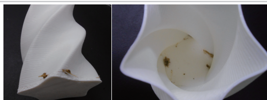
II. Printed object is polluted by different color filament
