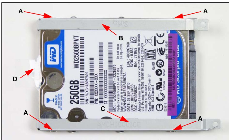
**Figure 3-13. HDD Module Brackets**
