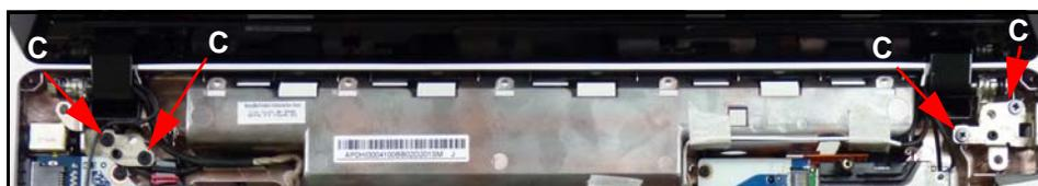
**Figure 3-57. LCD Module Hinge Screws**
