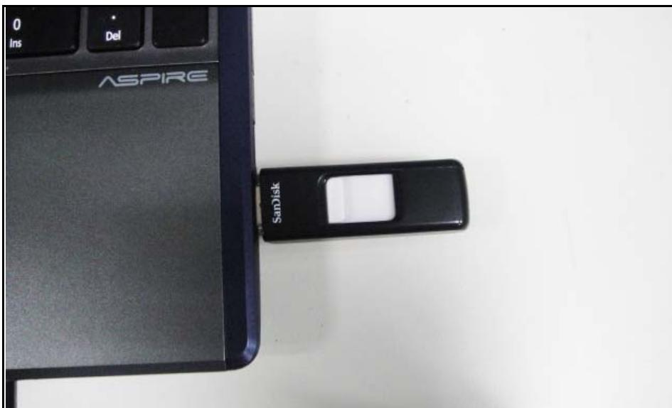
**Figure 5-14. Plugging in the USB HDD**
