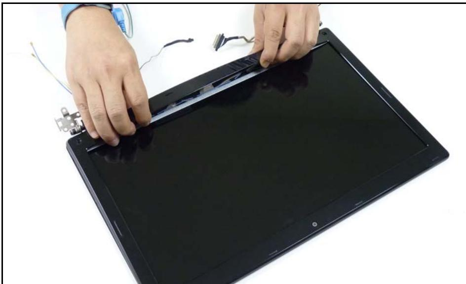
**Figure 3-61. LCD Bezel Removal**
