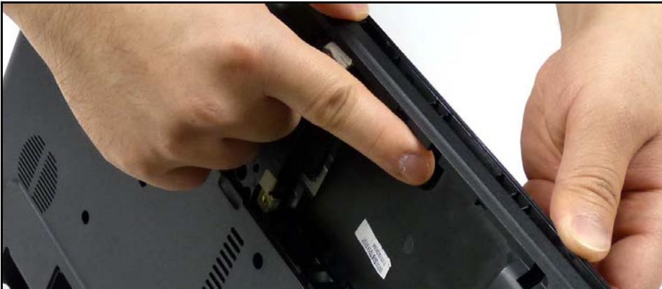
**Figure 3-24. Separating Upper Cover from Lower Cover**
