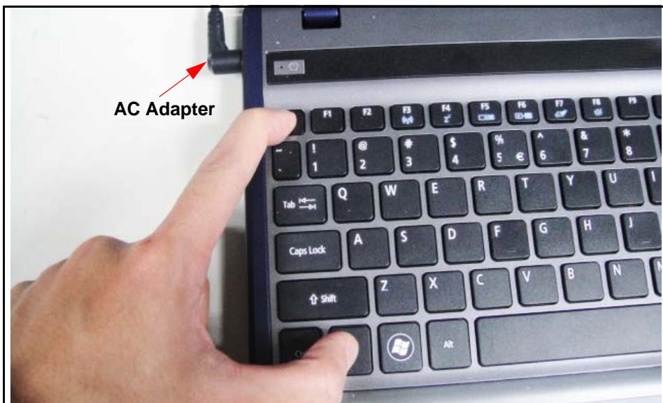
**Figure 5-16. Connecting AC Adapter (2 of 2)**
