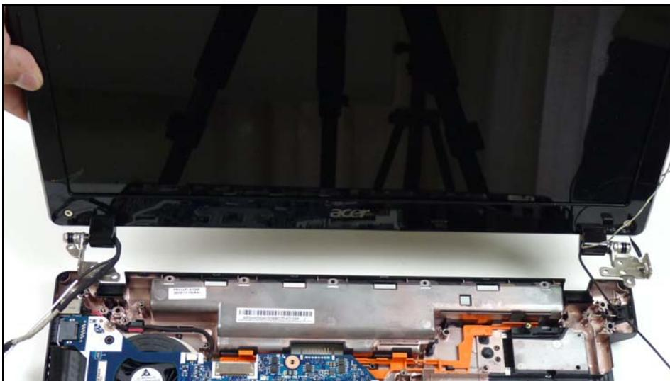
**Figure 3-58. Removing LCD Module**
