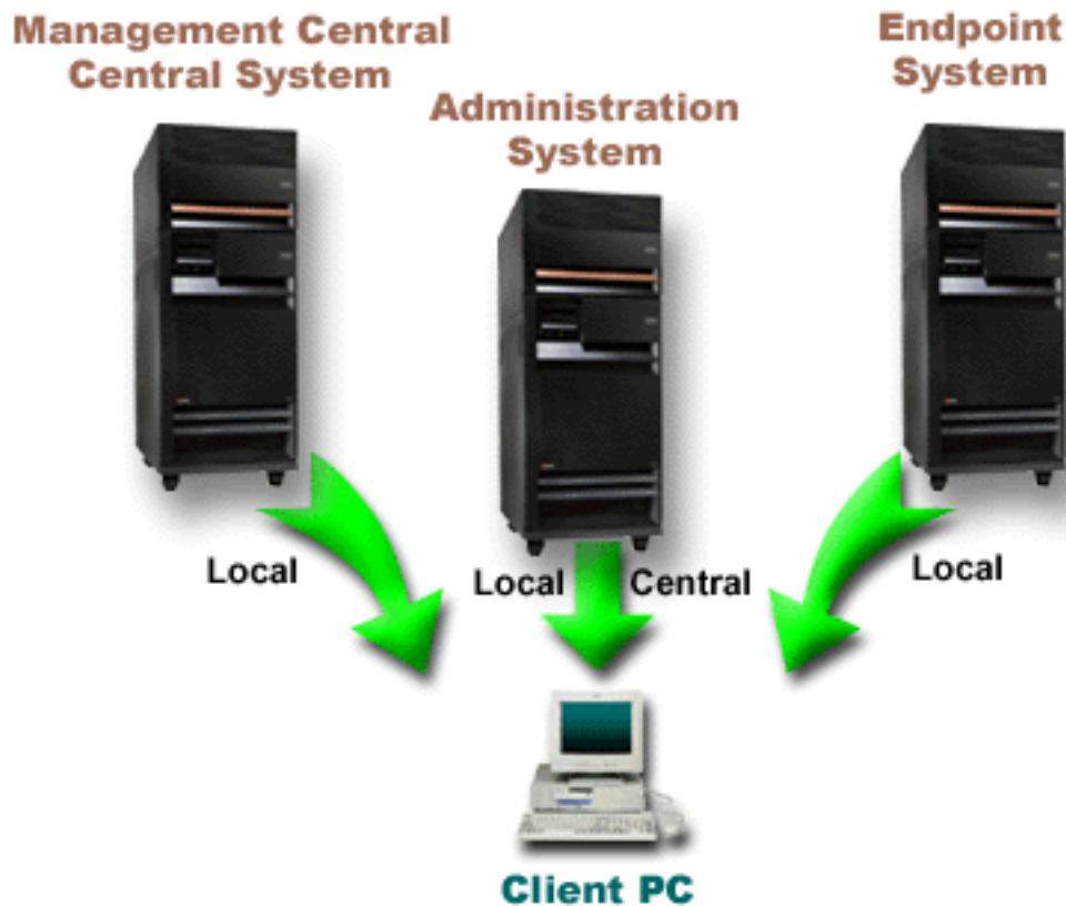
Figure 2. When a Client PC connects to a system, the Local Settings come from the system that you connect to. When you connect to an administration system, the Central Settings are sent to your Client PC from the administration system. This network does not change the function of Application Administration or Management Central.
