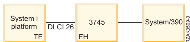
Figure 19. SNA direct connection to 3745 host controller
