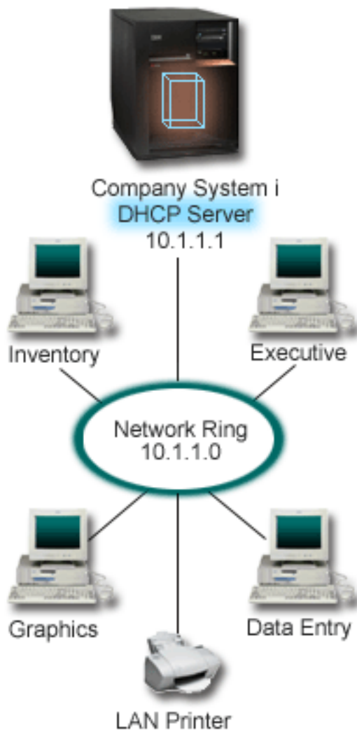
Figure 2. Simple LAN setup for System i model
