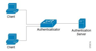
A network device can be either a client/supplicant, authenticator or both per port.
