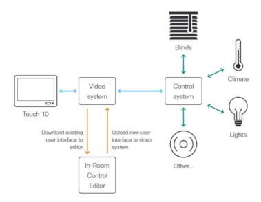
The graphical user interface can be designed by anyone, using the simple drag and drop GUI editor available on the endpoint's web interface. The editor can also be downloaded from the codec and used offline to later upload the design from a file.
