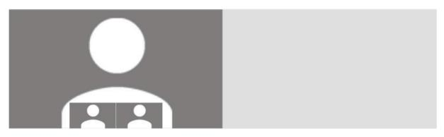
The above example shows a two-screen system in a conference where Multistream is not enabled. The endpoint is receiving only one transcoded stream from the Cisco TelePresence Server.
