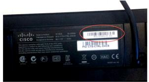
Identify the minimum software supported by using the TAN number with this table.
