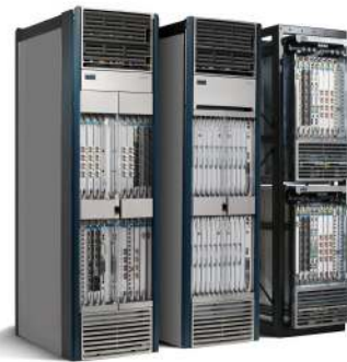
Cisco Carrier Routing System (CRS)
