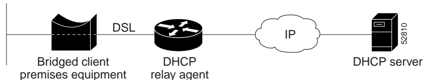
Figure 15 Network Topology Using ATM RBE and DHCP
