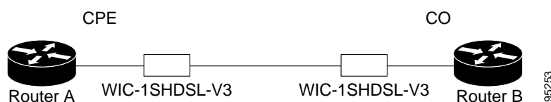
Figure 30 Basic Configuration for T1/E1 with a Back-to-Back Setup
