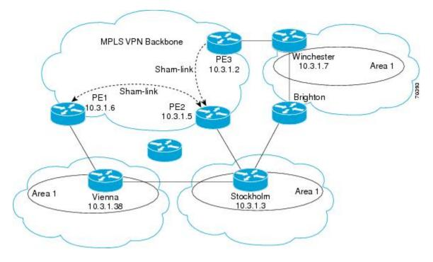
The following output shows the forwarding that occurs between sites from the standpoint of how PE-1 views the 10.3.1.7/32 prefix, the loopback1 interface of the Winchester CE router in the figure.
