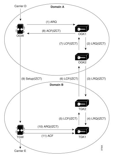
Figure 1 shows a simple inter-ITSP diagram of the IZCT flow.
