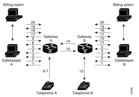
In this example, Telephone A is attempting to establish a phone call to Telephone B. The following numbered explanations correspond to the action taking place at each numbered reference in Figure 1.
