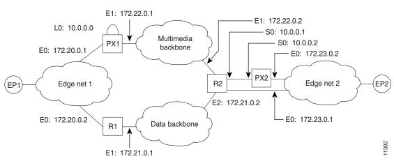
Figure 16 Edge Net 2 with Inside-Edge Proxy and No Subnetting
