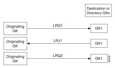
Figure 12 shows a call flow with the Sequential LRQ Enhancement feature when LRJ1 arrives after the delay timer has expired and after LRQ2 has been sent. If this occurs, the originating gatekeeper does not send LRQ3 and ignores LRQ2.
