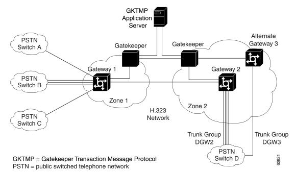
Figure 9 Topology of Routing Between Zone 1 and Zone 2
