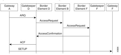
Figure 3 Address Resolution Using Border Elements
