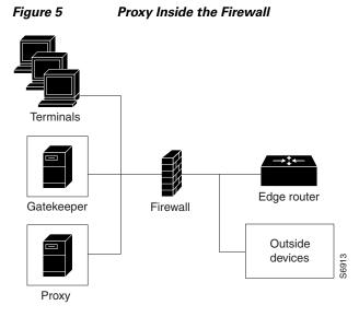
Because the gatekeeper (using RAS) and the proxy (using call setup protocols) are the only endpoints that communicate with other devices outside the firewall, it is simple to set up a tunnel through the firewall to allow traffic destined for either of these two endpoints to pass through.
