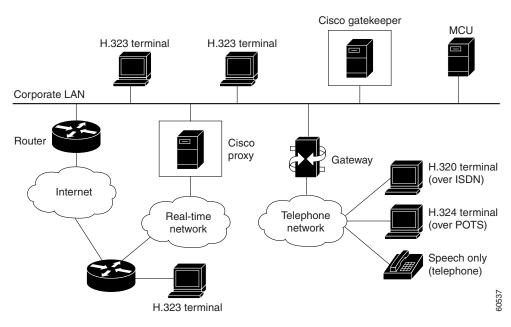
Figure 1 shows a typical H.323 network. Network components are described below.
