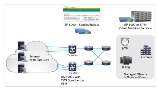
Figure 2. Key Peakflow Components
