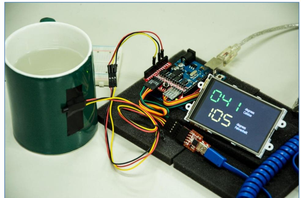
The LM35 temperature sensor is removed from the breadboard and connected to the Arduino Uno using a three-way cable.
