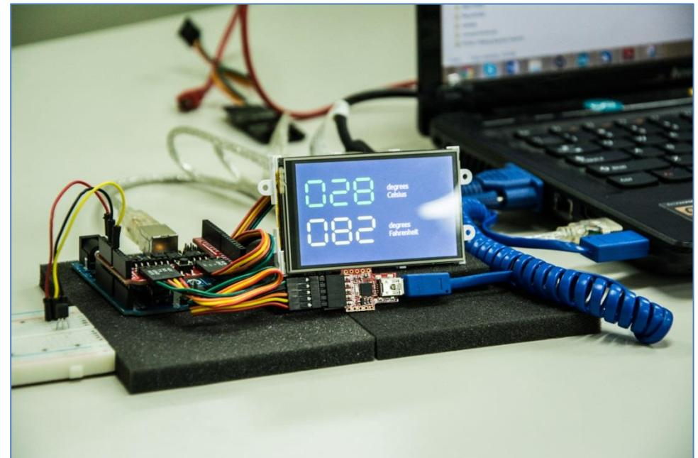
The uUSB-PA5 is used only to power the display.
