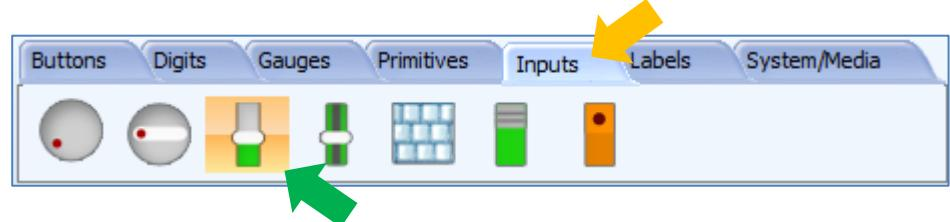
Click on the WYSIWYG screen to place the slider object. Drag the object to any desired location.
