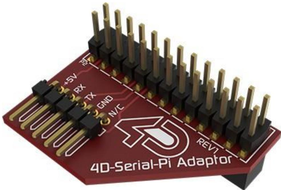
When using the 4D Serial Pi Adaptor, the display module is powered from the Raspberry Pi's 5V bus. The power supply therefore must be able to provide enough current to both the Raspberry Pi and the display module.
