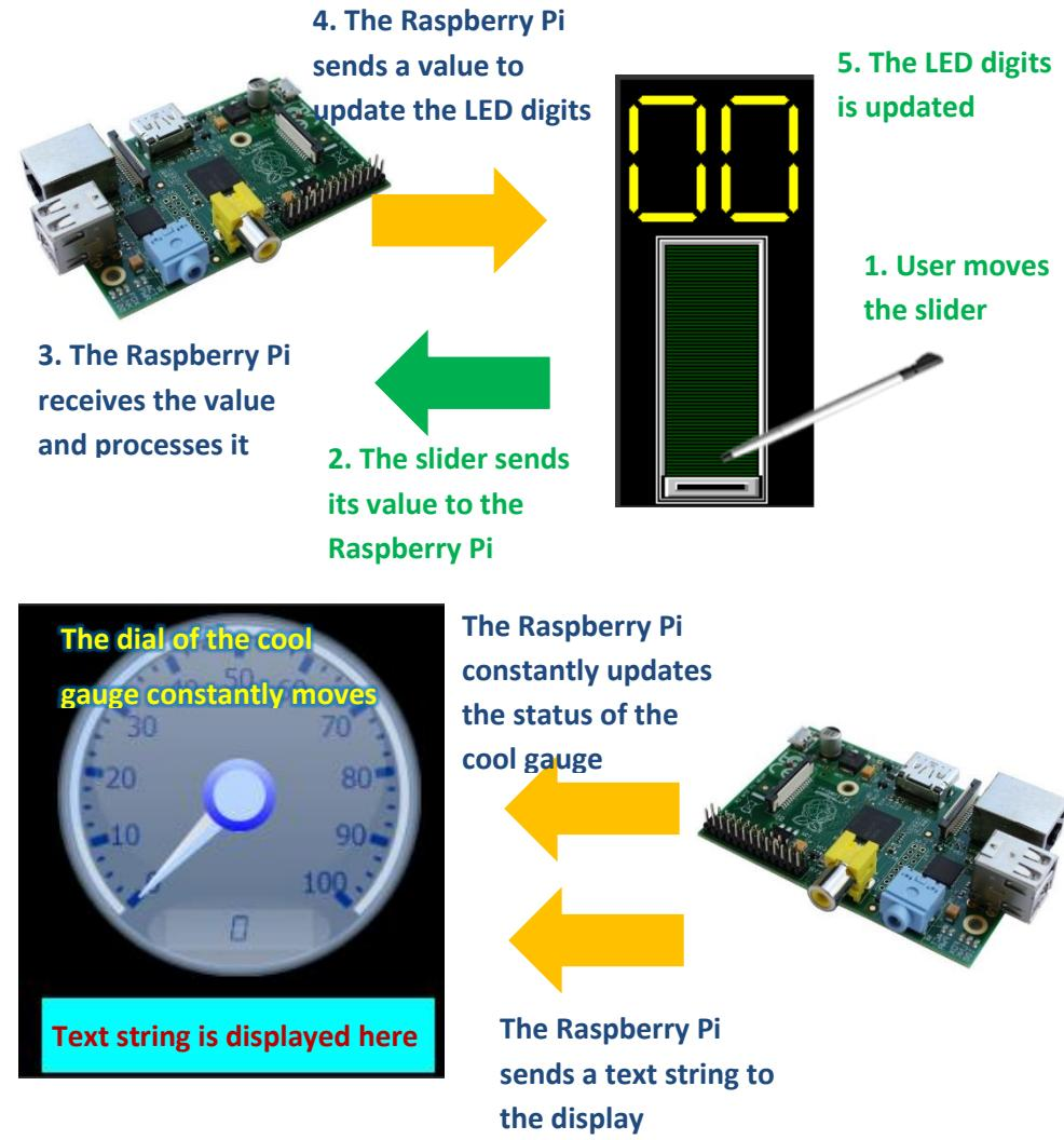
First the user creates a ViSi Genie program in the 4D Workshop IDE and downloads it to a 4D display module. On the other hand, a C program is created and is made to run on the Raspberry Pi. A library for the Raspberry Pi is provided by 4D Systems.
