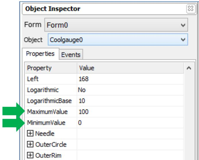
Feel free to experiment with the different properties. Take note of the maximum and minimum values. These determine the range of values that can be sent from the Raspberry Pi to the cool gauge. To know more about gauges, refer to [ViSi-Genie Gauges](#).
