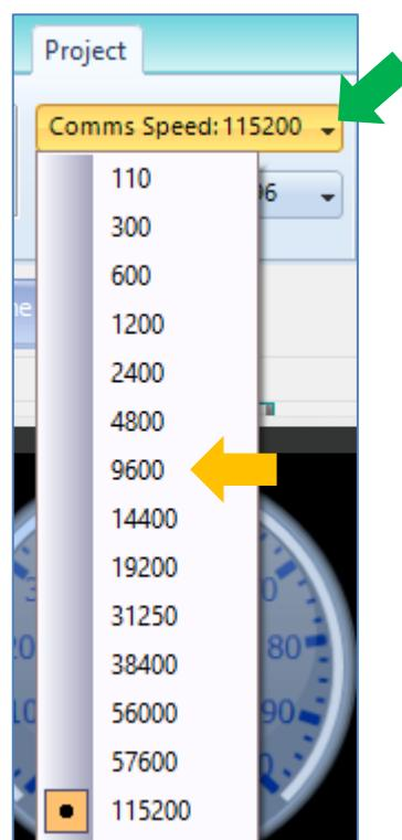
Choose the desired baud rate (9600 bps for instance) and download the program to the display module again. Now change the baud rate of the Raspberry Pi as well.
