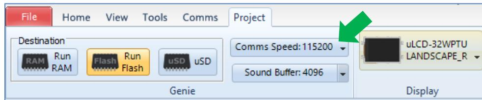
To change the baud rate of the ViSi Genie program, simply click on the drop down arrow.
