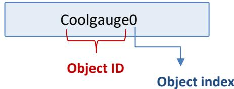
It is important to take note of an object's ID and index. When programming the Raspberry Pi, an object's status can be polled or changed if its ID and index are known. The process of doing this will be shown later.
