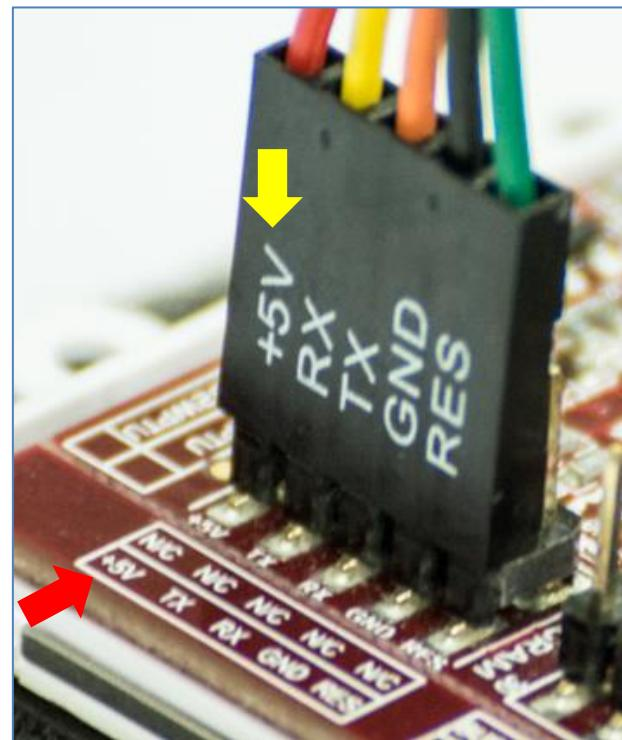
Check the orientation of the 5-way-cable-to-adaptor connection.
