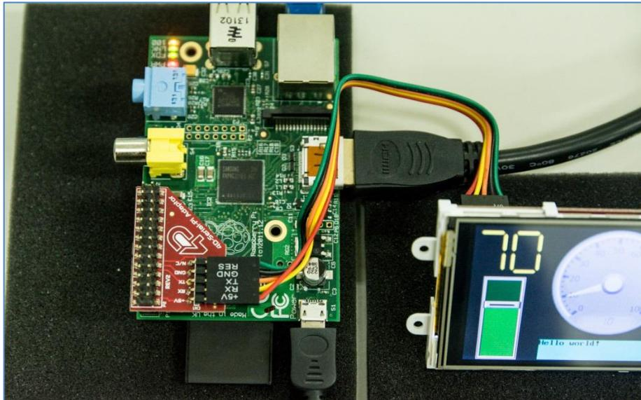
Check the orientation of the 5-way-cable-to-display-module connection.
