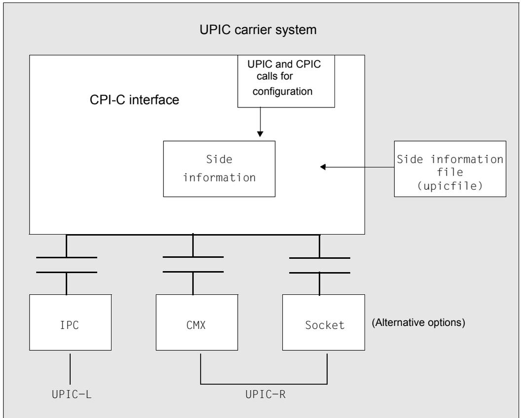
Figure 24: Configuration with and without side information file
