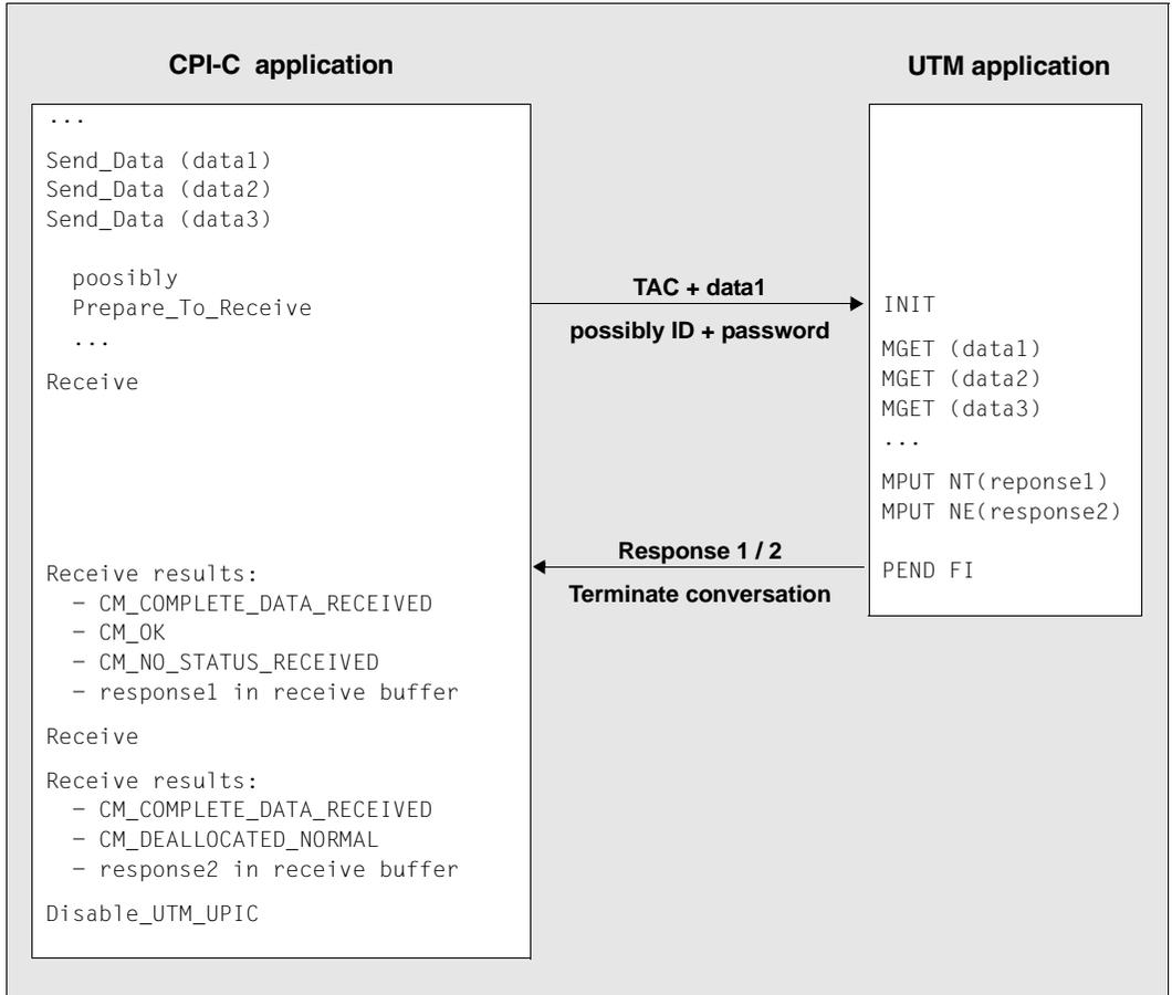
Figure 12: Single-step service with several Send/Receive calls
