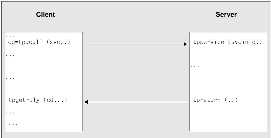
Figure 18: Asynchronous request response paradigm
