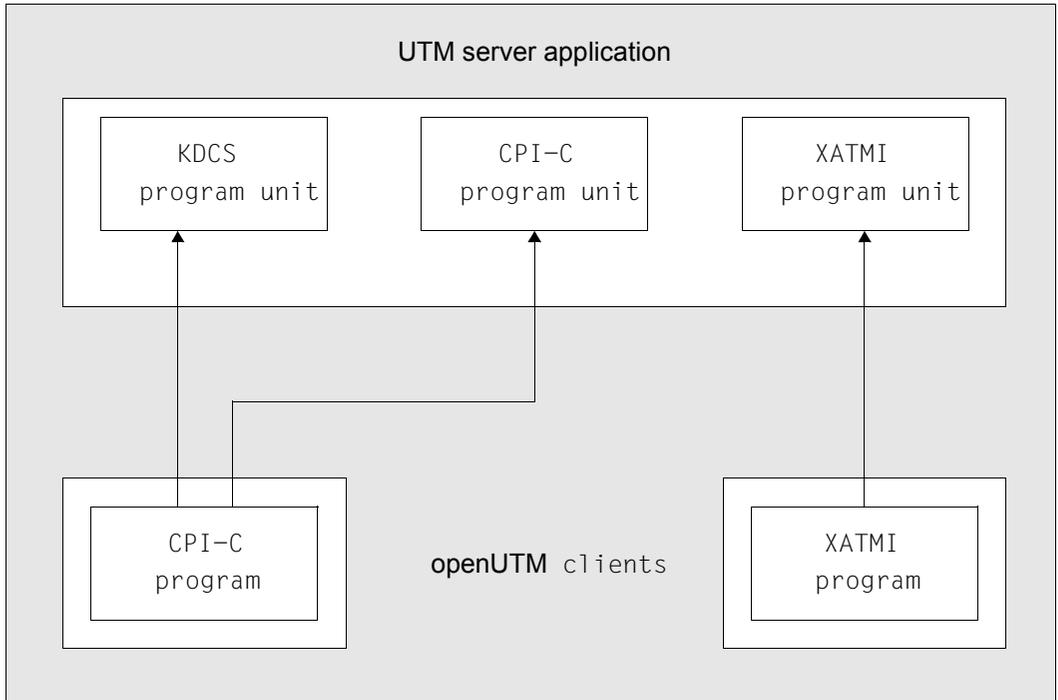
Figure 2: Interfaces between openUTM server and openUTM Clients
