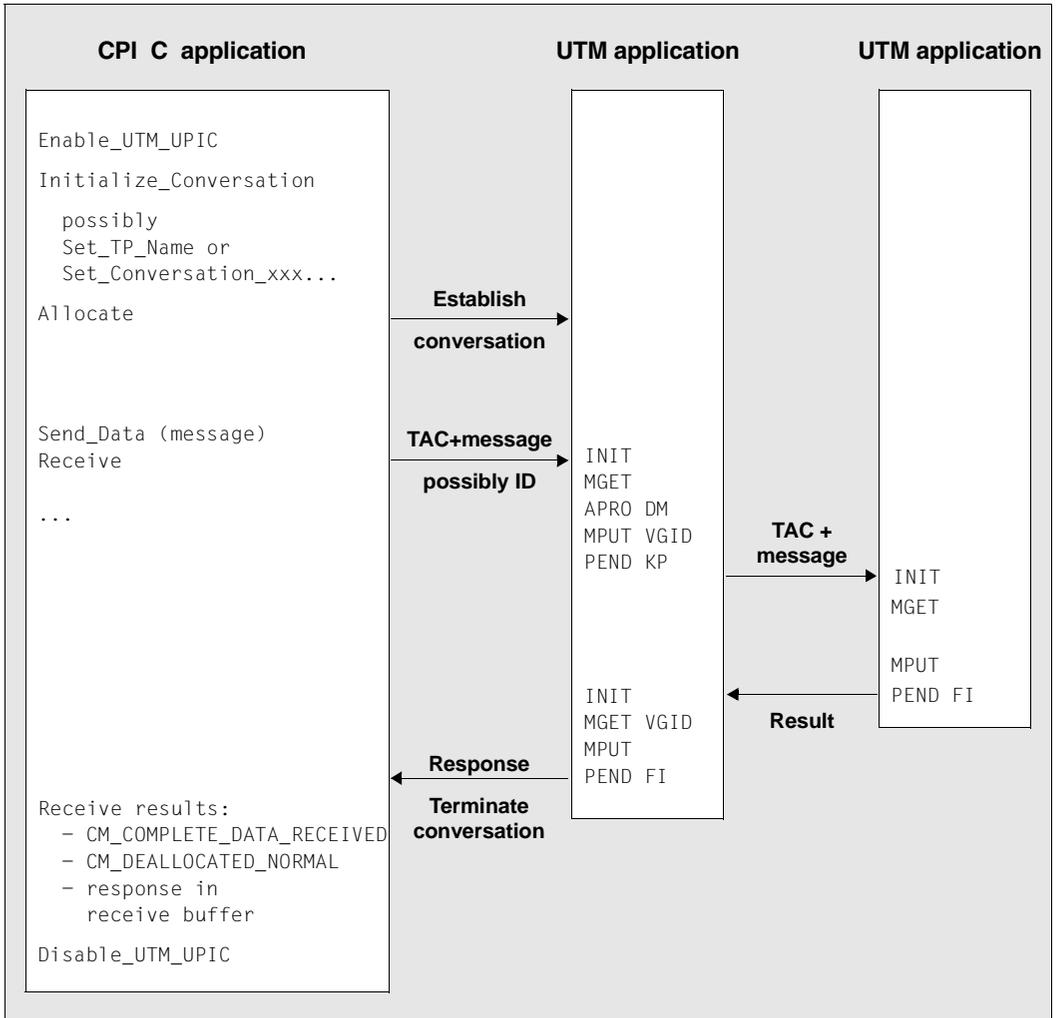
Figure 14: Multi-step service with DTP
