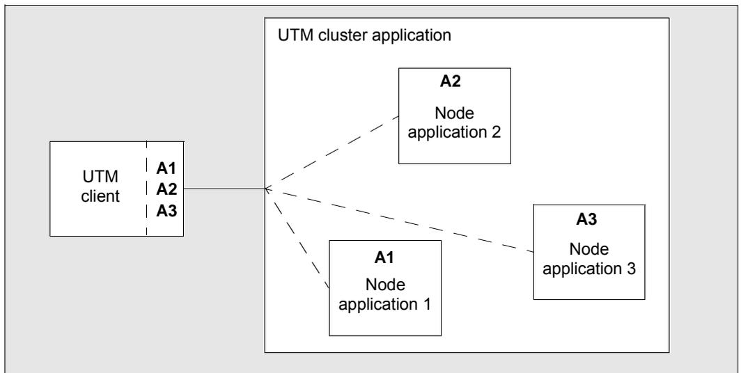
Figure 6: Communication with a UTM cluster application
