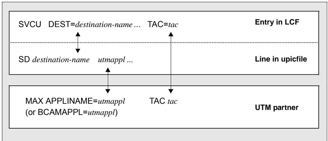
Figure 21: Conformance considerations when configuring server and client (operation without TNS)
